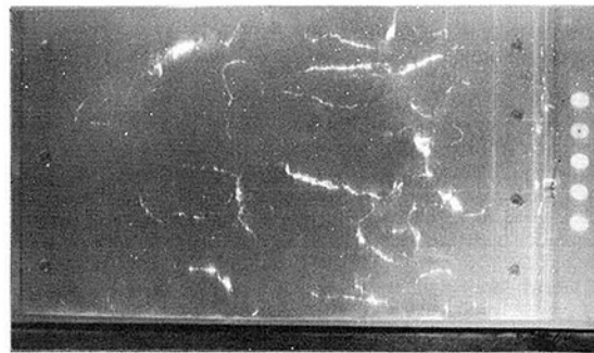
Fig. 4 Top view of cavitation behind the sharp-edged plate, Re_s = 2.28 \times 10^6 , \sigma_L = 0.601
